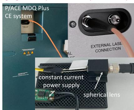
Direct LED coupling - machined aluminum adapter
