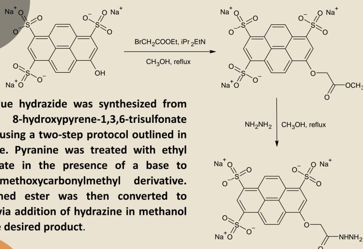
Cascade Blue hydrazide was synthesized from trisodium 8-hydroxypyrene-1,3,6-trisulfonate (pyranine) using a two-step protocol outlined in the scheme. Pyranine was treated with ethyl bromoacetate in the presence of a base to afford *O*-methoxycarbonylmethyl derivative. The obtained ester was then converted to hydrazide via addition of hydrazine in methanol to yield the desired product.
